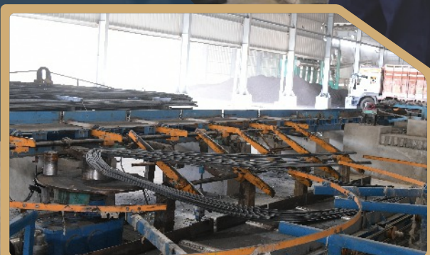
Bending, Stacking and Dispatch System
